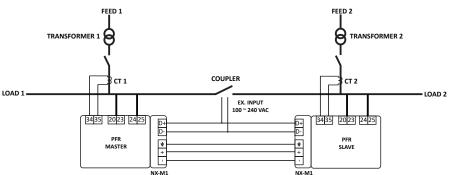
Nх-м1 Diagram 2 - Example of PFRs operate in two feeds system
