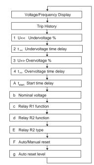
Figure 3: Display mode when pressing Reset/Mode
