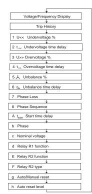
Figure 4: Display mode when pressing Reset/Mode
